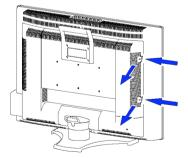
Remove the back plate at the back of the TV as shown on the illustration opposite.
